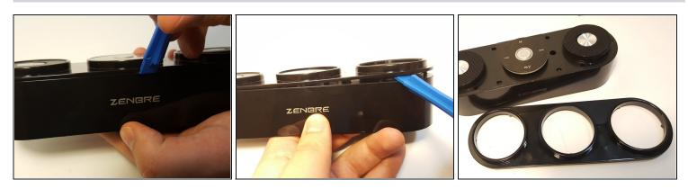
• Remove the top plastic cover by prying around the edges with an iFixit opening tool.
