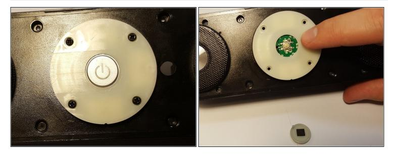
• Pick up the center power button and remove it. Place it in a safe location.
