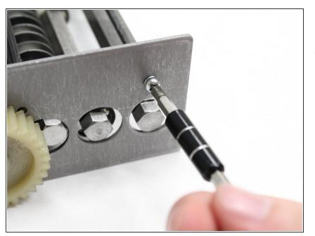
Remove the 15 mm Phillips #1 screw located on the metal side plate of the shredding unit.
