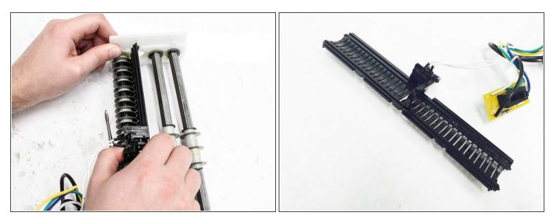
Unhinge the sensor clamp from the blade by pushing with your thumb and pull the sensor away from the plastic side piece with the other hand to detach the activation sensor from the entire shredding unit.
