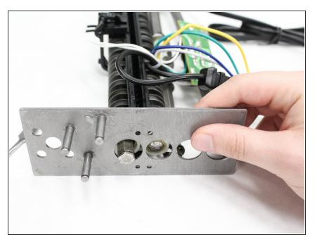
• Remove the metal side piece from the shredding unit.
