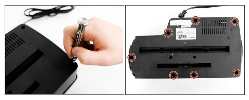
The unit head needs to be switched to the off position and unplugged before any disassembly.
