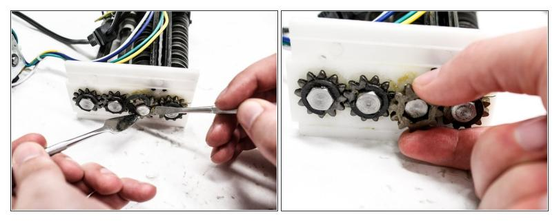
• Remove the washer from the gear second from the right using two metal spudgers. Place one spudger on each of the open ends of the washer. Push down with both spudgers at the same time to pop the washer off the gear.
