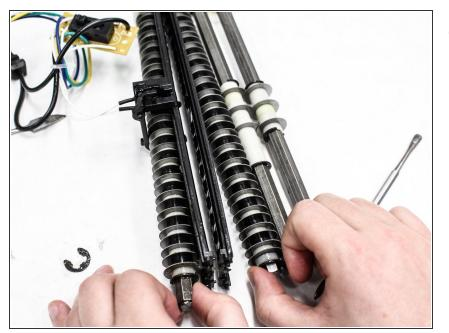
Remove the middle blade from the plastic side piece by pulling it away from the sensor. The blade will fall away from the other attached parts of the unit.
