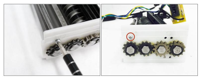
• Remove the 15 mm Phillips #1 screw located on the plastic side plate of the shredding unit.
