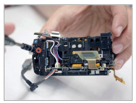
Orienting the camera such that the right side is facing you, remove the single 5.5 mm Phillips #00 screw from the start button.
