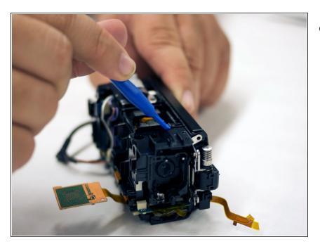
Use your blue plastic opening tool to disconnect the lens assembly from the hull.
