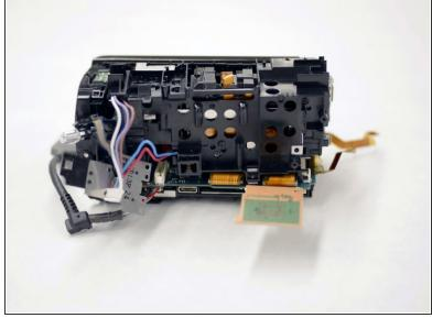
Orienting the camera such that the right side is facing you, remove the wire harness connecting the lens assembly to the motherboard using your tweezers.
