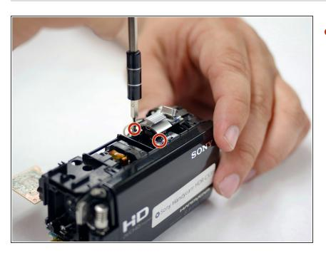
With the back of the LCD screen facing toward you, remove the two 5.5 mm Phillips #00 screws from the zoom button.
