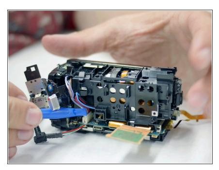
Use your blue plastic opening tool to move the wires out of the way.
