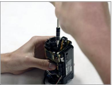
Remove the three 5.5mm Phillips #00 screws holding the lens in.
