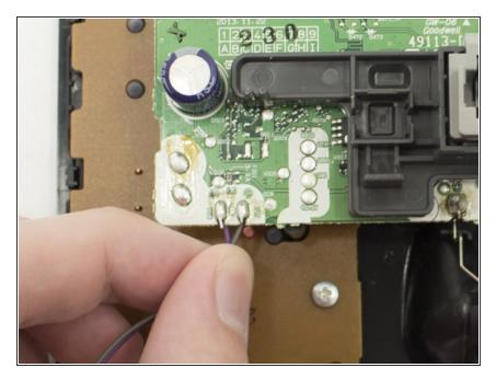
The faulty power port can now be detached from the device from its contact points. If soldering has been successful, removal should require minimal effort.
