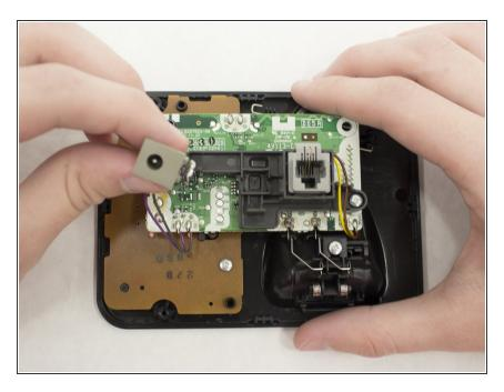
Now that the device has been opened, the power port can easily be removed from its resting point.
