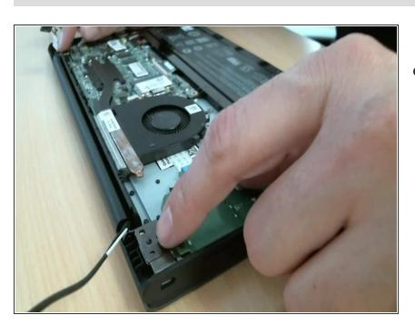
To separate the chromebook chassis from the LCD assembly, pull the chassis upward while holding the LCD assembly against the table. This will cause both hinges to move upward which will then allow enough space for the chassis to be detached from the LCD assembly's hinge joints. (See video)
