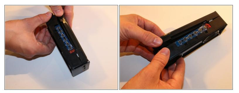
• Pull apart the two faces to separate the back panel from the front face plate.
