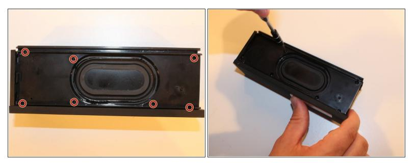
On the back panel (Opposite to the side containing the two speakers), Use the Philips head PH1 to remove all 7 screws (Screws: Head PH1, Length 7cm).
