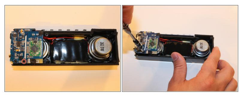
Remove the single screw holding the motherboard to the front panel (Screw : Head PH1, Size .5 cm)
