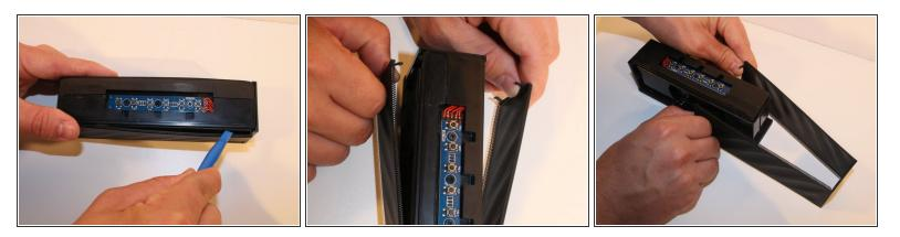
There are four prongs on the grill in the corners, closest to the power button switch. Use the plastic
