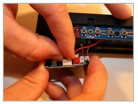
Disconnect the Button Panel plug (Largest of the Plugs, it can be traced back to the button panel easily)
