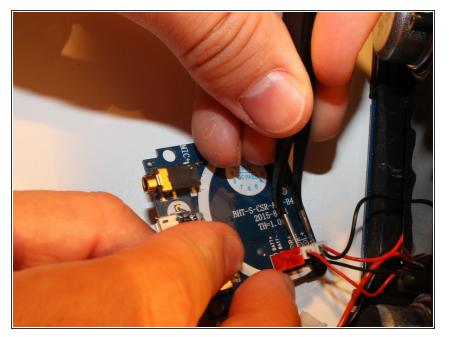
Use the tweezers to push down on the two safety prongs on the plastic switch. Then Disconnect the two Speaker plug connections by hand (Two Smaller Plugs)
