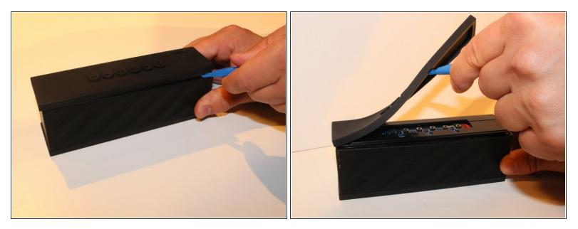
Using Blue Plastic opening tool pry the top rubber cover, then using the same tool remove the bottom panel
