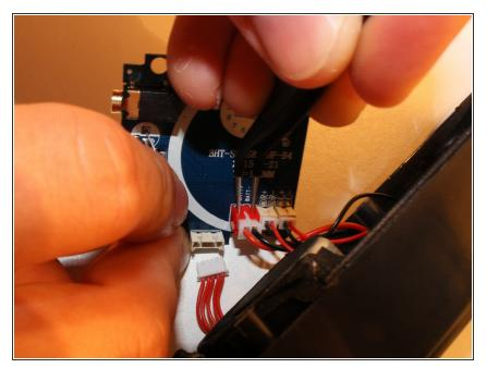
Use the tweezers to push down on the safety prongs on the plastic switch. Then Disconnect the Power Wire plug by hand (Red medium),
