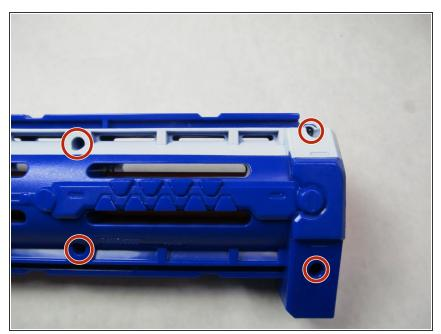
• Disassemble the barrel assembly by removing four 8mm Phillips screws from the blue barrel housing.
