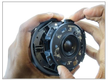
• The speaker should now easily come off with a firm grip on the OnHub device and pull.
