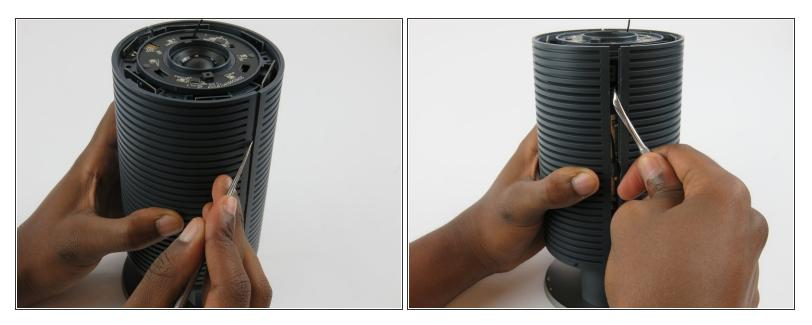
• Once the two screws are removed from the base, it is time to split the casing apart.
