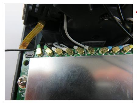
Make sure to carefully pull the tape style wire furthest to the left that is held by glue.
