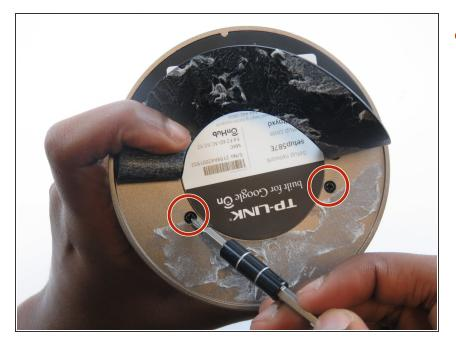
Remove the two 12mm screws under the base of the OnHub by using a #1 Phillips head screwdriver.
