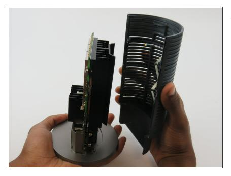
Once unclipped, you can slide the two casing halves apart, and remove the casing.
