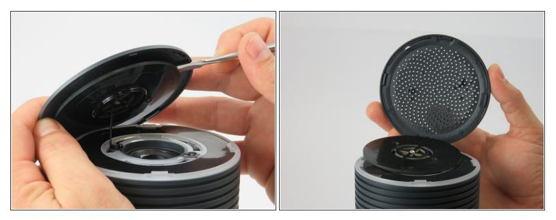
• Using a metal spudger, carefully remove the congestion-sensor antenna by undoing the two clips.
