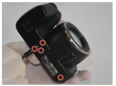
Remove the M3 x 4mm screws from the bottom of your device as indicated by the picture. using the Philips Head J0 Screw Driver Bit.
