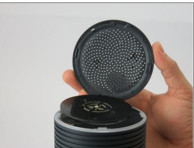
Using a metal spudger, carefully remove the congestion-sensor antenna by undoing the two clips.
