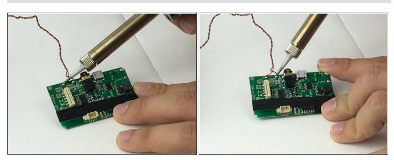
Desolder the wires that connect the LED to the motherboard.
