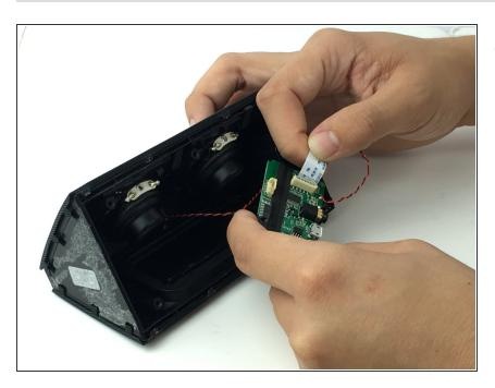
Unplug the thin white cable connected to the buttons.
