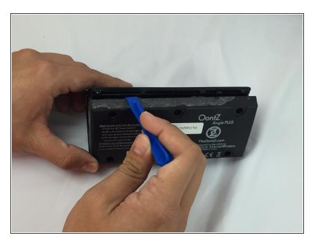
Carefully pull apart the bottom plate and the top plate, using the blue plastic opening tool.
