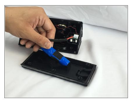
Separate the battery from the bottom plate and set the bottom plate aside.
