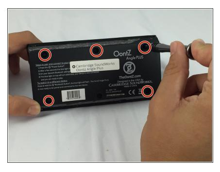
Unscrew the five 11.5mm Phillips screws on the bottom plate.
