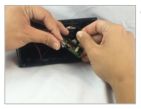
Unplug the wires that connect the speakers to the motherboard.
