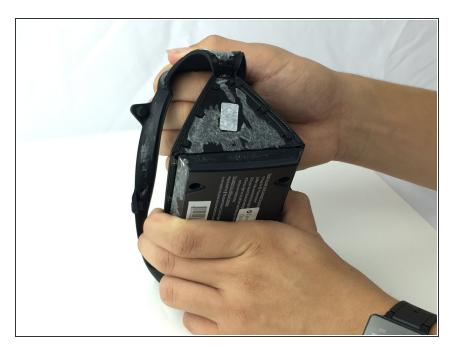
Carefully pull off the casing covering the ends.
