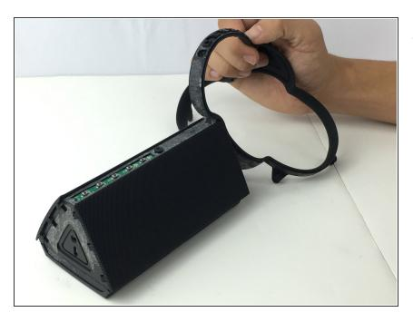
Slowly remove the casing from the top of the device.
