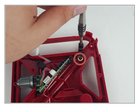
Remove the Philips #1 screw, securing the FM radio antenna to the case.
