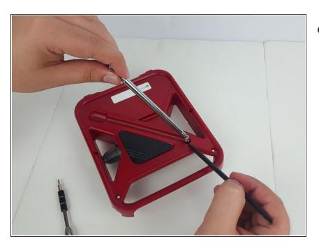
From the back of the device, gently pull the antenna out of the device case.
