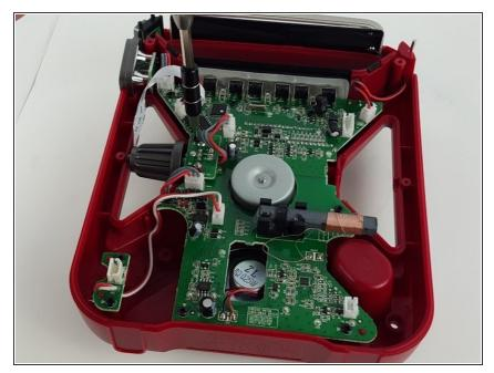
Remove the two 1 cm Phillips #0 screws that secure the tuning dial panel to the motherboard.
