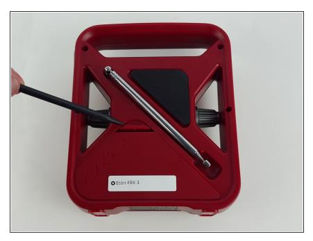
Pull the plastic tab on the battery compartment cover panel to loosen it, then pull the panel off.
