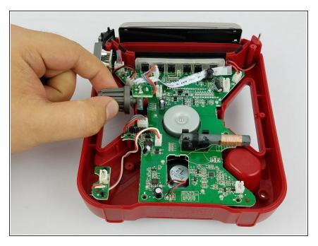
Gently lift the dial upwards to remove it.
