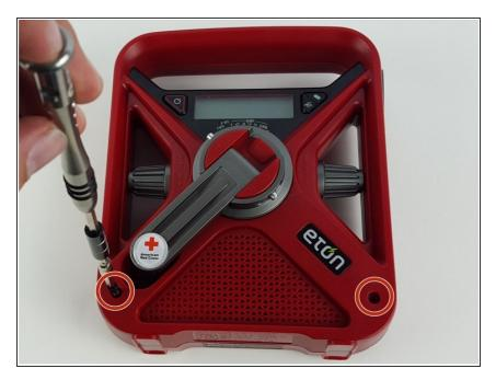
On the bottom of the device case's face are two T10 screws. Use a T10 Torx screwdriver to remove the two screws.
