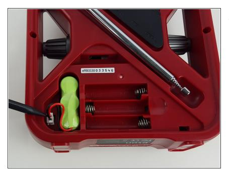
Disconnect the battery pack wires from the device and remove the battery pack.
