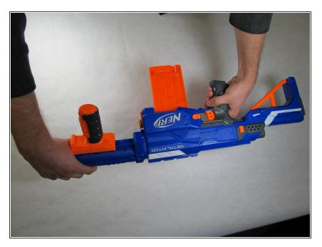
While holding the blaster, rotate the barrel assembly in the counterclockwise direction and pull away from the blaster.
