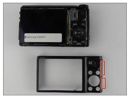
Once the screws are removed, use the blue opening tool to open the back case from the sides - it should come off easily.
