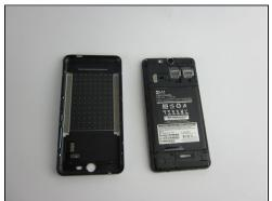
Remove the back case using plastic opening tool.
