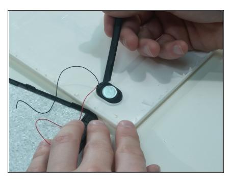
• Use the plastic spudger to remove speaker from the back panel.
