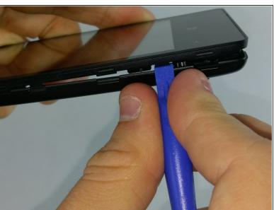
Using a plastic opening tool, pry apart the inner back case apart from the rest of the phone, starting at the top and prying while going around the phone.
