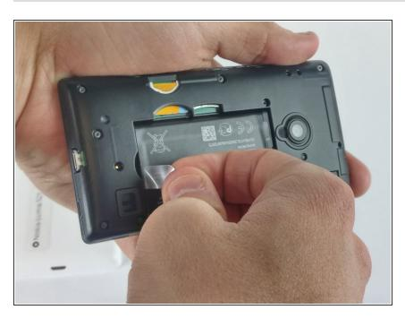
Once the cover has been removed, the battery will be visible. Grab the plastic tab and pull it to remove the battery from its place. If there is no plastic tab, use the plastic opening tool to pry the battery loose.
