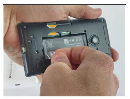
Once the cover has been removed, the battery will be visible. Grab the plastic tab and pull it to remove the battery from its place. If there is no plastic tab, use the plastic opening tool to pry the battery loose.
