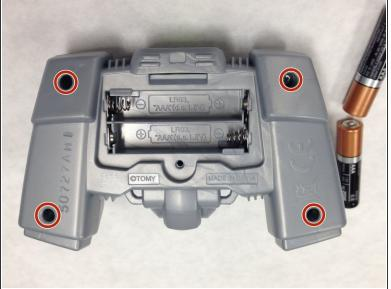
Using the Hex 4 socket and PH #0 bit, remove the four 8 mm screws on the panel.
