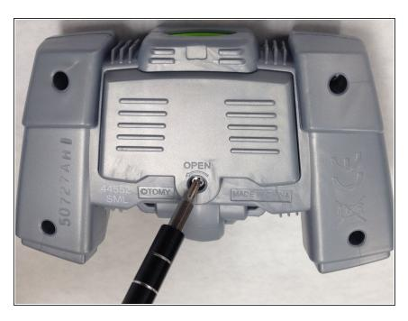
Remove the screw on the battery lid.
