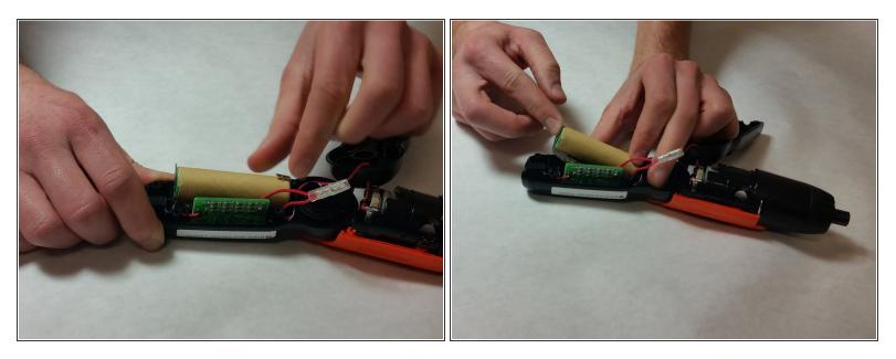
• Using pliers or your fingers, remove the leads off of the battery.
