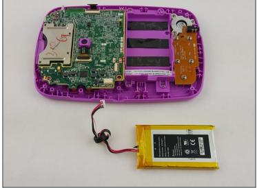
• Pry the battery gently off of the plastic platform with an opening tool.
