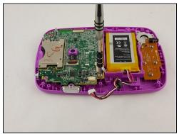
Remove the three 6 mm phillips head screws holding the motherboard to the display assembly.
