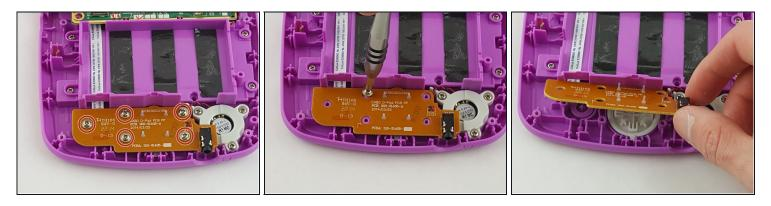
• Unscrew the five 6.0 mm phillips head screws from the board containing the audio jack and directional pad.
