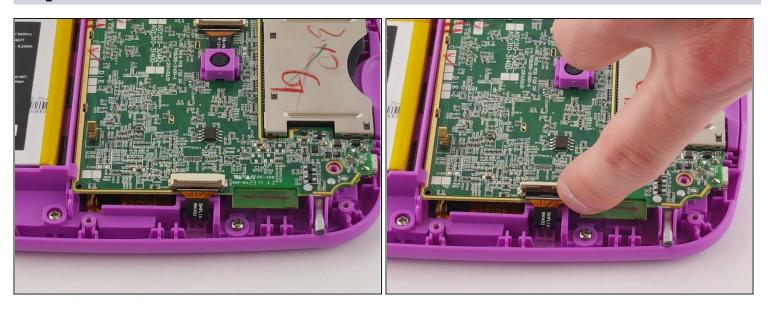
• Unplug the front facing camera cord with an opening tool to free the top of the motherboard.
