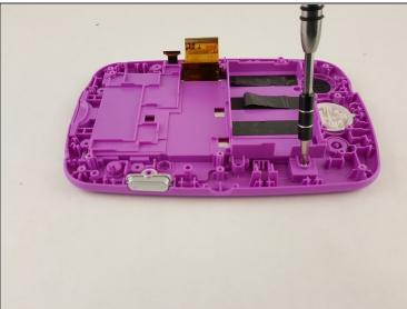
Unscrew the eight 6.5mm Phillips #0 screws from the plastic casing.
