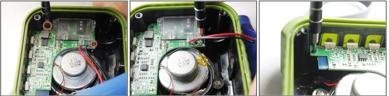
**⚠ Remove all three Phillips screws which holds the motherboard to the base using a PH00 Phillips screwdriver.**
