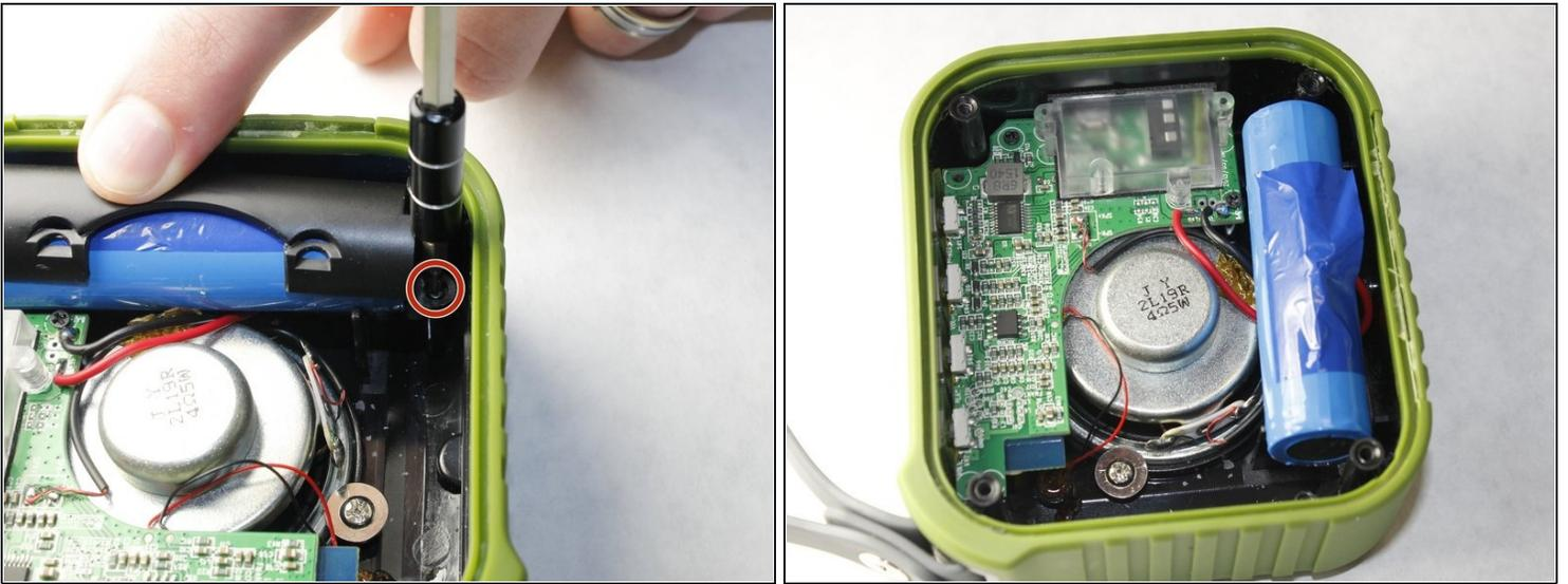
⚠ Remove the two Phillips screws which hold its battery casing on the housing using a PH00 Phillips screwdriver.
