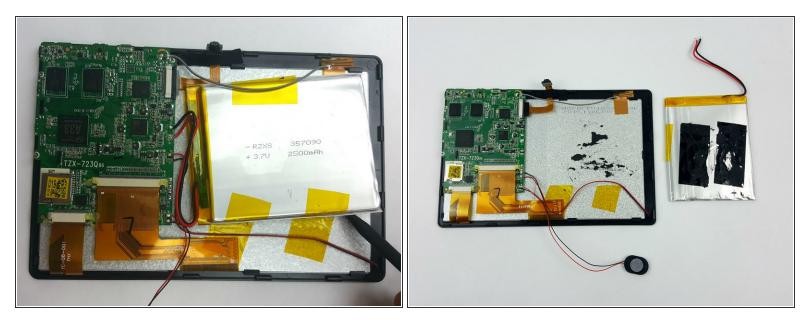
Insert plastic spudger under the battery and slide back and forth, separating the battery from the case.
