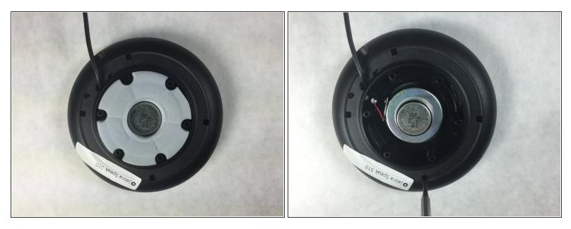
• Remove the back plate and the grey foam underneath.
