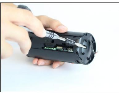
Using the driver adapter, first insert the #4 socket into the driver; followed by the #1 Philip's head bit in order to reach the three 13.0 mm screws.
