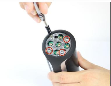
Remove the eight 7.0 mm Phillips #1 screws on both sides of the JBL Flip 2.
