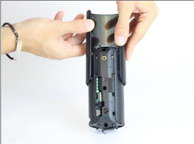
Expand the metal casing and carefully slide it off the speaker.
