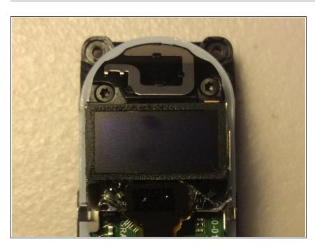
You can Then pull out the Screws from around the Screen
