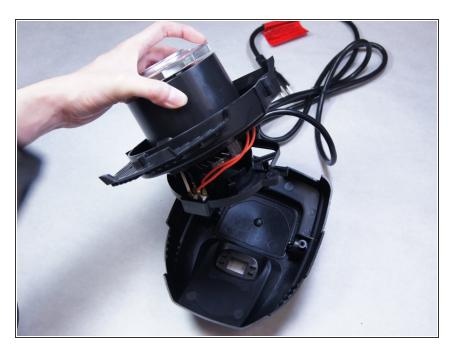
Separate the power unit assembly from the cover.
