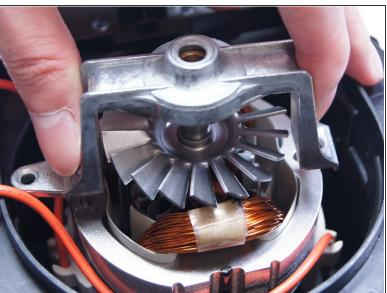
Remove the motor bracket.
