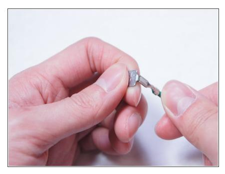
Separate the clip from the green wire and transfer it to the replacement motor.
