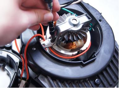
Use a Torx T15 driver to unscrew the two screws securing the metal motor bracket.
