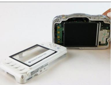
Using a plastic opening tool, gently remove the back cover from the camera.
