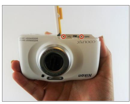
Remove the two screws located above the HDMI and USB logos that are inside the camera's battery compartment using a JIS000 screwdriver.
