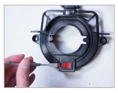
Use a spudger to pry up and remove the red switch from the housing.
