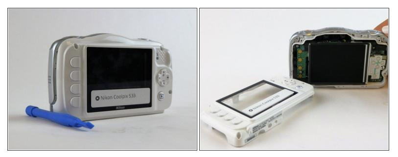
• Using a plastic opening tool, gently remove the back cover from the camera.
