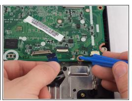
Use a plastic opening tool to carefully lift the white hinge up on the touchpad cable connector, and gently remove the cable from the motherboard.
