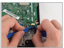
Use two plastic opening tools to grip each side of the connector for the speaker cable and gently pull the cable from the motherboard.
