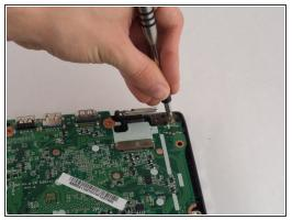
Remove three 6.2 mm Phillips #1 screws that attach the motherboard to the laptop casing.
