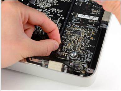
Pull the vertical sync cable connector out of its socket on the LED driver board near the top left corner of your iMac.
