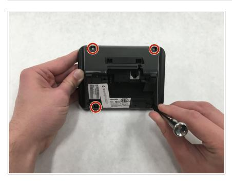
To open the main docking station, you'll need to remove four 11 mm Philips #0 screws.
