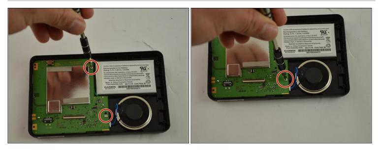
• Use your T5 Torx screwdriver and unscrew the two 5.0 mm screws on the motherboard.
