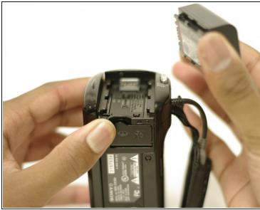
Using your right index finger and thumb, pull the battery toward you and then away from the camera.
