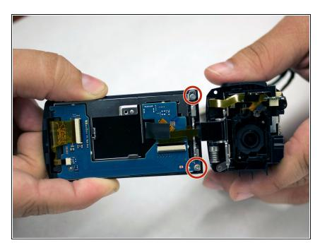
Remove the two silver-colored 4.5 mm Phillips #00 screws from LCD board.
