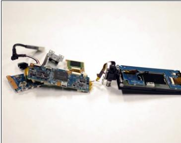
• Using your left hand to hold the camera, remove the motherboard from the camera's hull using your right thumb and index finger.
