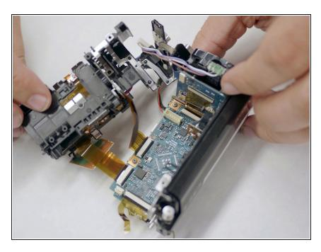
Pull the lens assembly out from inside the camera's hull using your hands.
