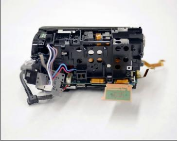
• Orienting the camera such that the right side is facing you, remove the wire harness connecting the lens assembly to the motherboard using your tweezers.
