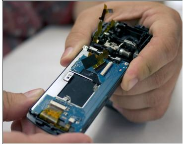
With tweezers, remove the ribbon cable that is connecting the LCD screen board to the motherboard.
