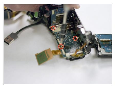
Remove the three 5.5 mm Phillips #00 screws attaching the motherboard to the camera's hull.
