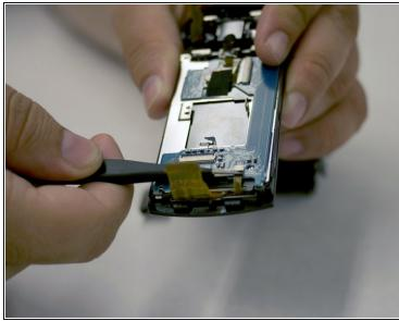
• Using metal tweezers, remove the two ribbons connecting the LCD board to the screen.
