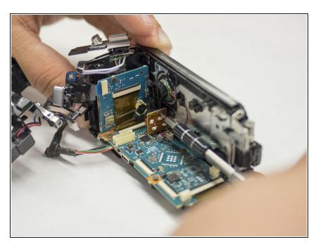
• Remove the 5.5 mm Phillips #00 screw above the microphone jack.
