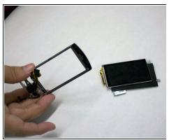
• The LCD screen and all of its components are free. Unravel them and replace parts as needed (main board, screen, metal fixture, etc.)
