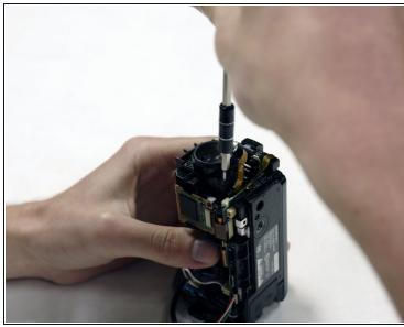
• Remove the three 5.5mm Phillips #00 screws holding the lens in.
