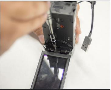
• Remove the single 3 mm Phillips #00 screw from inside of the hinge of the LCD panel.
