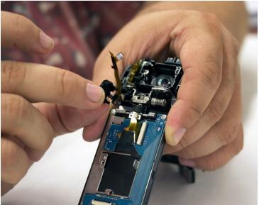
Remove the hinge enclosure from the back of the LCD screen using the blue plastic opening tools.
