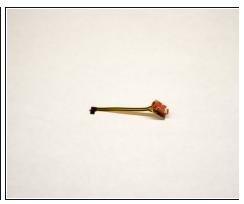
Using your left hand to hold the camera, remove the microphone jack with your right thumb and index finger.
