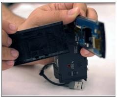
• Using the plastic opening tools , remove the back panel from the LCD screen.
