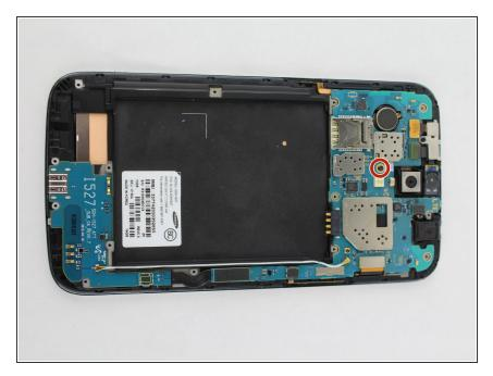
Remove the 2.55 mm Phillips #000 screw from the motherboard panel.
