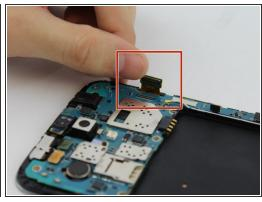
Remove the connector clips on motherboard.
