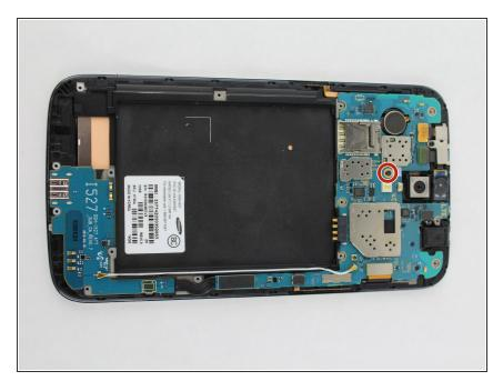
Remove the 2.55 mm Phillips #000 screw from the motherboard panel.
