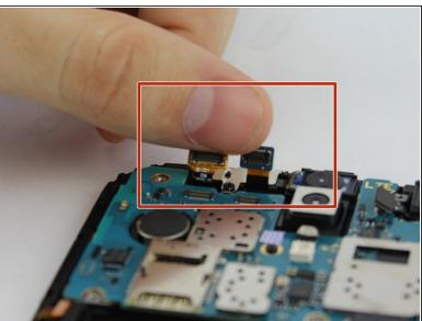
Remove the final motherboard connectors.
