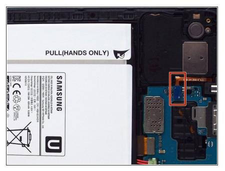
Use the spudger to disconnect the 3.5mm headset jack's flexible cable connector.
