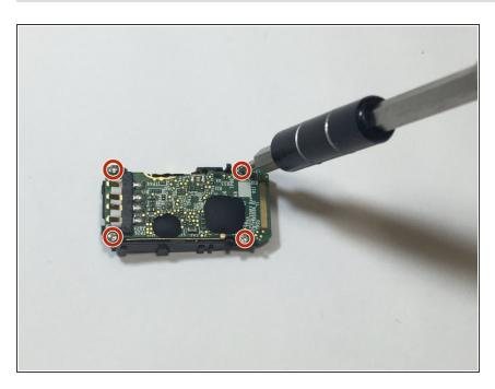
Remove the four highlighted screws from the motherboard using the Philips screwdriver.
