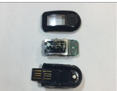
After the cover had been removed, use the metal spudger tool to remove the body of the device from the casing.
