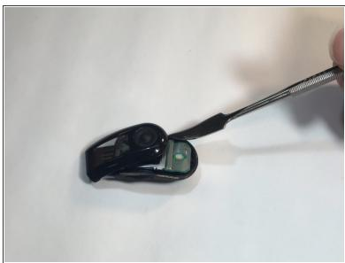
Finish the disassembly of your NikePlus Sportband by utilizing the metal spudger tool on the short edge to pry the external body pieces apart.
