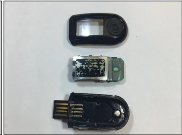
After the cover had been removed, use the metal spudger tool to remove the body of the device from the casing.
