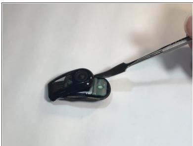
Finish the disassembly of your NikePlus Sportband by utilizing the metal spudger tool on the short edge to pry the external body pieces apart.
