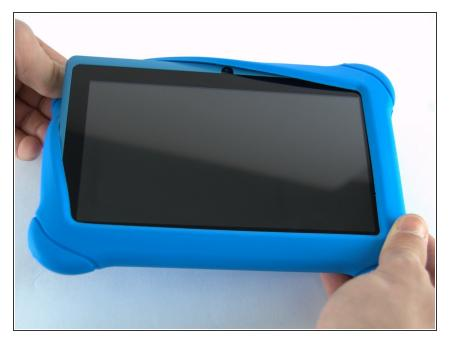
Use your thumbs to gently pry the silicon case away from the tablet starting at one of the corners. Once the first corner is separated the other three corners should slip off easily.
