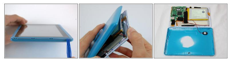
• Use the plastic opening tool to pry the back off the tablet. Work your way around the edges. Once you have one side open you can slowly unsnap the rest of the case and use the tool as needed.
