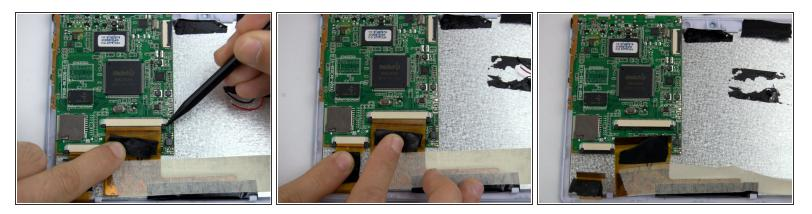
• Using the tip end of the spudger, slide back the black clips on the side of the right ribbon connection.
