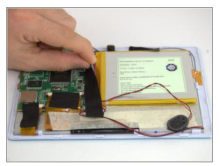
• Pull back the tape to expose the wires that are attached to the battery.
