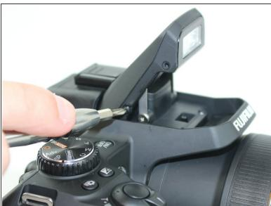
Remove the 4 screws from the flash casing.
