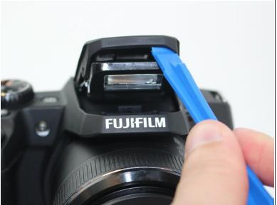
Pry the edges off of the flash casing, and pull it off of the camera.
