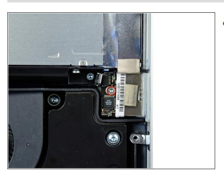
Remove the single 8 mm T8 Torx screw securing the SD board to the outer case.
