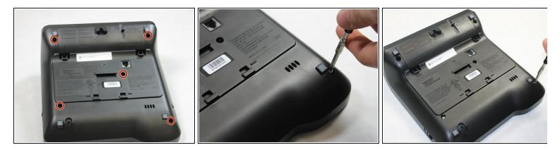
• Remove five 9.5 mm Phillips #1 screws from the back panel of the phone.
