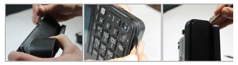
• Slide the metal spudger into the crack and continue around to the front panel of the phone.
