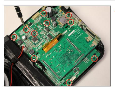
Remove (10) screws (10 mm) with a PH1 screwdriver on the display board.
