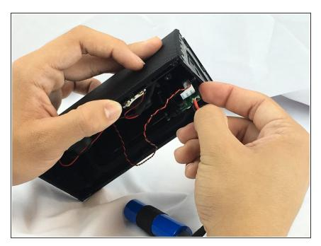
With some force, push the motherboard straight in toward the center of the device.
