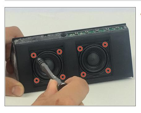
Unscrew the eight screws holding the speakers in place.
