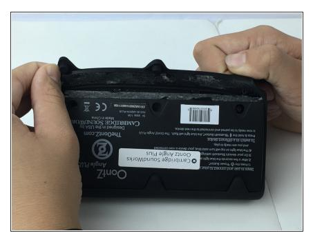
Starting from the screw covers, remove the front and back casing of the device.
