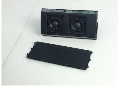
Finally, bend the speaker cover upward and it will slide out.
