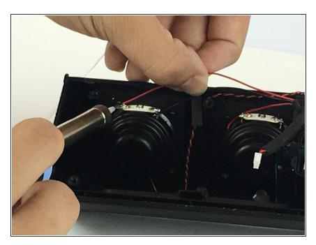
Desolder the the wires connected to the back side of both speakers.
