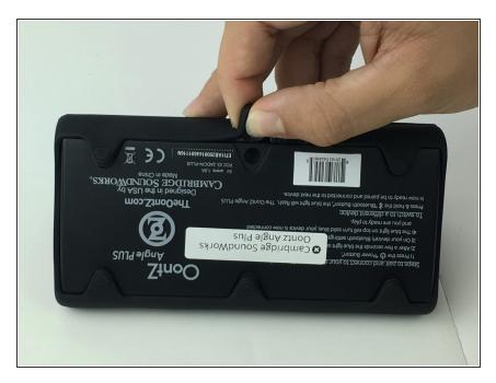
Remove the six screw covers from the bottom of the device.
