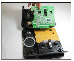
• Lift the top level Motherboard in order to get to the lower level Motherboard.
