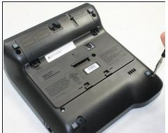
• Remove five 9.5 mm Phillips #1 screws from the back panel of the phone.
