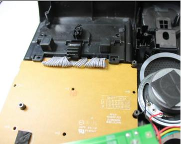
• Unscrew five 5.6 mm screws on the lower level Motherboard.
