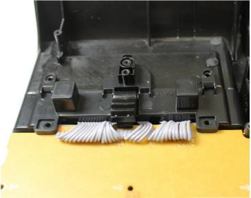
Unscrew the 5.6 mm screw on the clip behind the Screen as shown.
