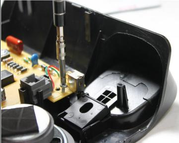
Unscrew five 5.6 mm screws on top level, yellow motherboard.
